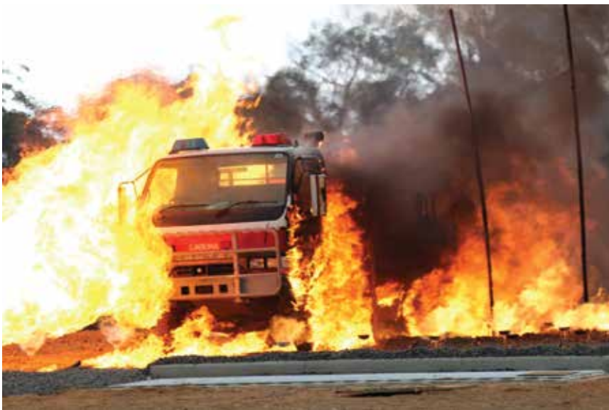
CSIRO burnover testing a firefighting vehicle to support development of crew protection systems at the NSW Rural Fire Service Hot Test Fire Facility at Mogo in NSW. Photograph courtesy of CSIRO.
