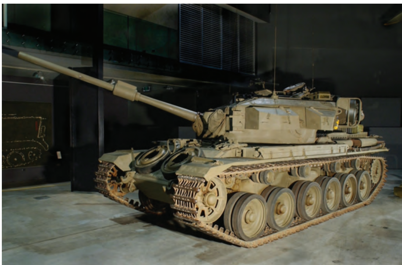
Centurion Mk 5/1 Main Battle Tank with damage to the hull near the right-hand exhaust shroud, possibly sustained in active service. AWM Accession Number: REL/16440.001.
